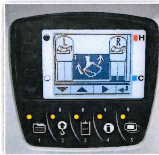
Max. oil flow setting (AUX1 and optional AUX2)
