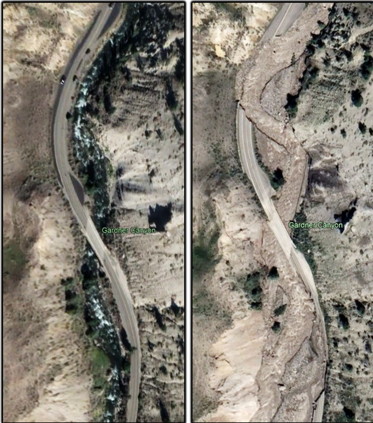
Caption: Highway 89 S between Gardiner, Montana, and Mammoth, Yellowstone National Park, Wyoming, south of Rescue Creek trailhead is washed away by the Gardner River 2022 flood. The image on the left is from 2019 while the image on the right is from 2022.
