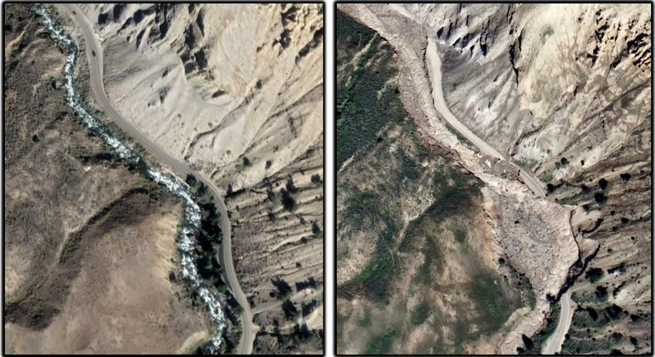
Caption: Highway 89 South between Gardiner, Montana, and Mammoth, Yellowstone National Park, Wyoming, at the 45 th parallel is washed away by the 2022 Gardner River flood. The image on the left is from 2019 and the image on the right is from 2022. Source: Google Earth Imagery.
