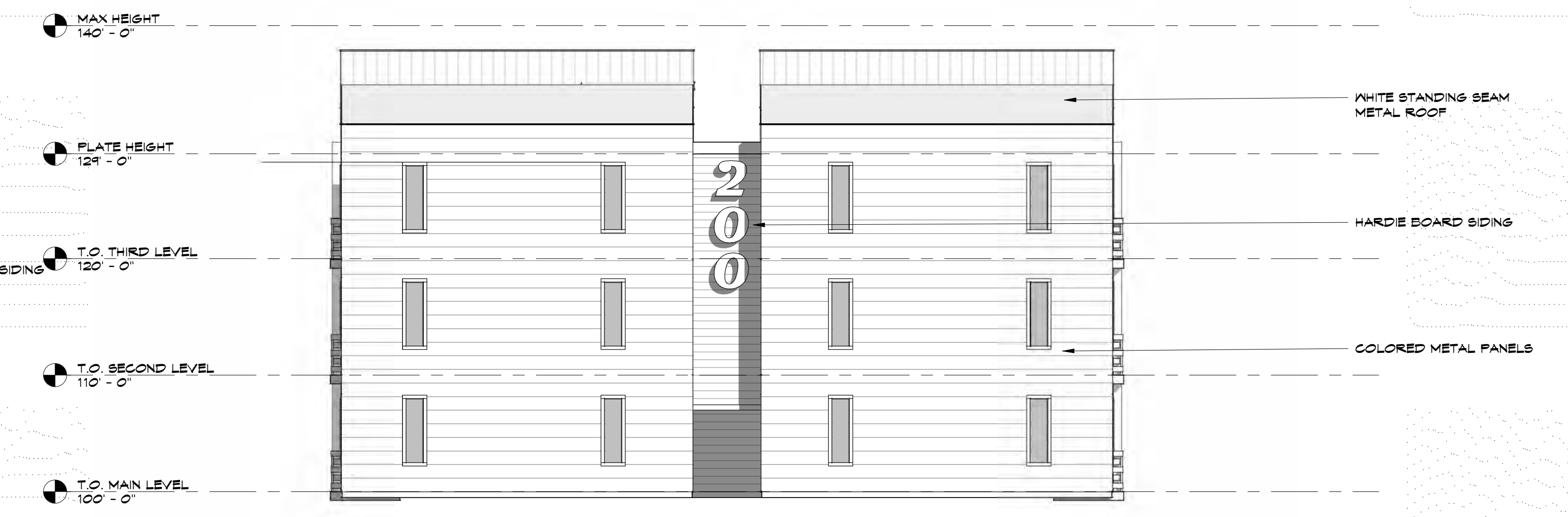
3 ELEVATION - 36 UNIT BUILDING 1/8" = 1'-0"
