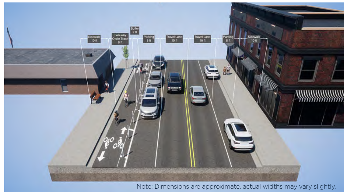
Proposed Cycle Track (Pilot Project) Configuration on 2nd Street (Looking South)
