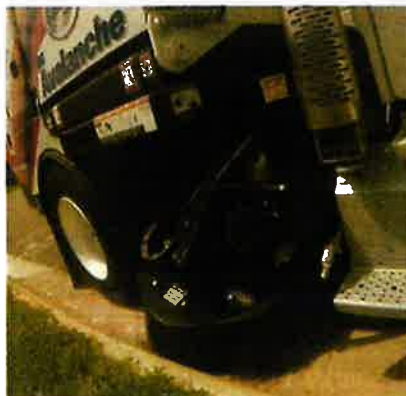
9" Diameter Side Broom(s) with Outer Broom Extension Override.
