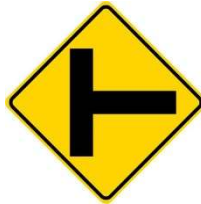
Figure 4. Side Road Advanced Warning Sign (MUTCD W2-2R)
