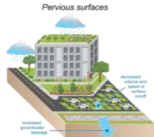
Pervious 'soft' surfaces (green roofs, rain gardens, grass paver parking lots, and infiltration trenches) decrease volume and speed of stormwater runoff. The slowed water seeps into the ground, recharges the water table, and filters out many pollutants and sediment before they arrive in downstream waters.
