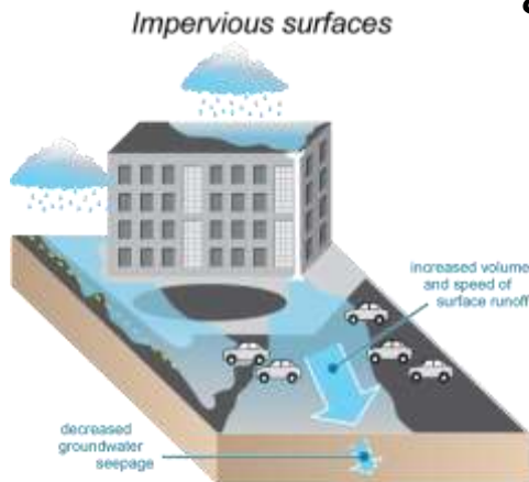
Impervious 'hard' surfaces (roofs, roads, large areas of pavement, and asphalt parking lots) increase the volume and speed of stormwater runoff. This swift surge of water erodes streambeds, reduces groundwater infiltration, and delivers many pollutants and sediment to downstream waters.
