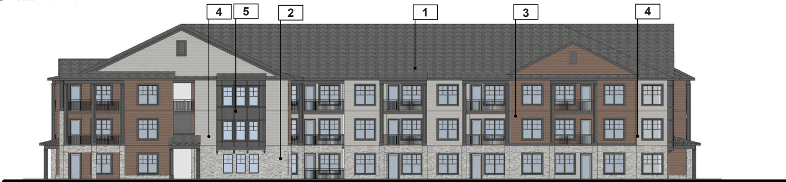
4 Elevation: Building Type C - "L" Rear Scale: 1/16" = 1' 0"
