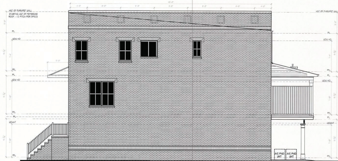
2 Right Side Elevation - WYNFIELD & WILLMINGTON SCALE: 1/4" = 1'-0"
