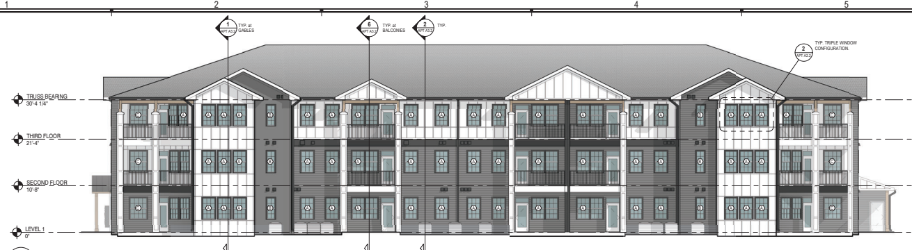
A LONG ELEVATION - BUILDING A APT A2.1 1/8" = 1'-0"
