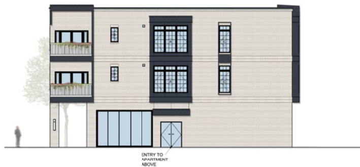
2 ELEVATION - MIXED-USE BUILDING - BLOCK D - WEST A503 SCALE: 1/8" = 1'-0", WHEN PRINTED IN 24"x36" SHEET SIZE
