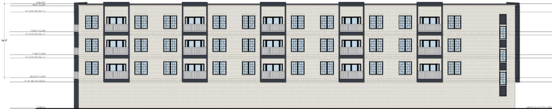
2 ELEVATION - APARTMENT BLOCK B - SOUTH A302 SCALE: 1/8" = 1'-0", WHEN PRINTED IN 24"x36" SHEET SIZE
