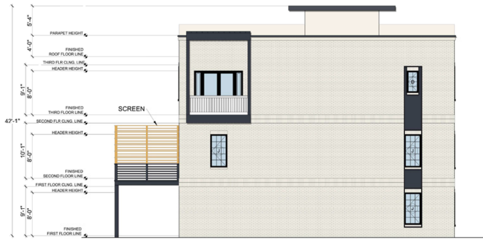
1 ELEVATION - TOWNHOMES - BLOCK C - EAST A403 SCALE: 3/16" = 1'-0", WHEN PRINTED IN 24"x36" SHEET SIZE
