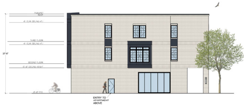
1 ELEVATION - MIXED-USE BUILDING - BLOCK D - EAST A503 SCALE: 1/8" = 1'-0", WHEN PRINTED IN 24"x36" SHEET SIZE
