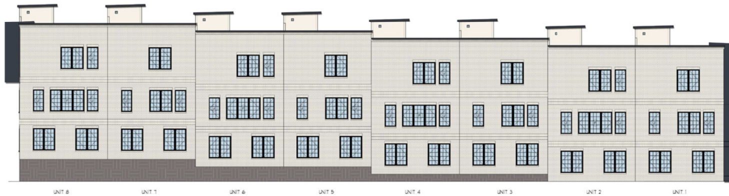
2 ELEVATION - TOWNHOMES - BLOCK C - NORTH A402 SCALE: 1/8" = 1'-0", WHEN PRINTED IN 24"x36" SHEET SIZE
