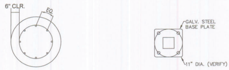
7/A.2 Light Pole Mounting Detail Scale: 3/4" = 1'-0"
