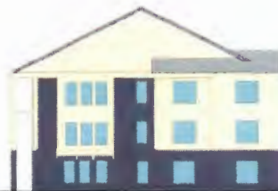
Right Side Elevation - Building Type A - Material Designation Total Façade: 1445 SF Brick: 819 SF Percentage: 56%
