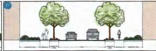
ENTRY DRIVE SECTION AT MULTI-FAMILY AND COMMERCIAL
