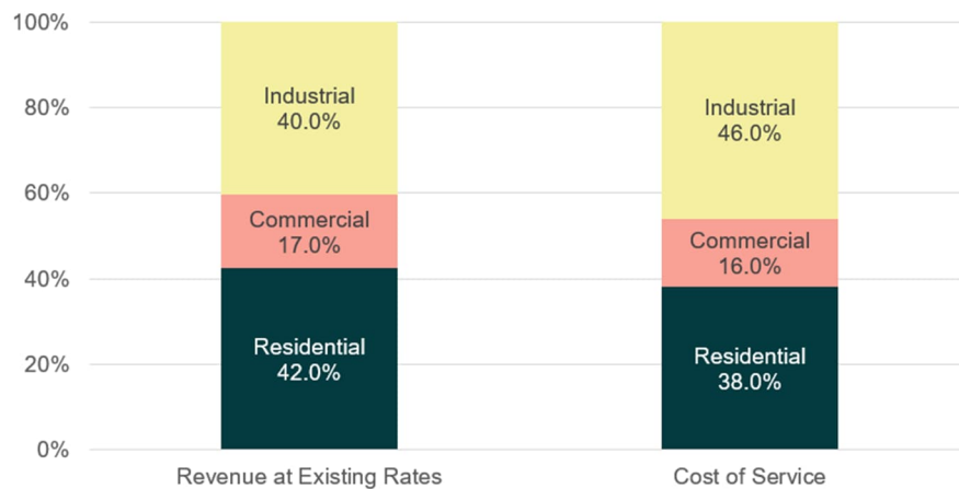
Figure 5: Allocation of Water Utility Costs Under Current Rates Compared to the Allocated Cost of Service
