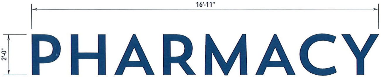
5 ILLUMINATED CHANNEL LETTERS - REMOTE SCALE: 3/8" = 1'-0" 34.0 SQ. FT.
