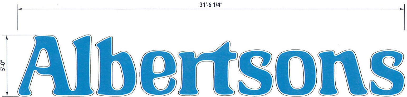
2 CUSTOM ILLUMINATED CHANNEL LETTERS - REMOTE SCALE: 1/4" = 1'-0"
