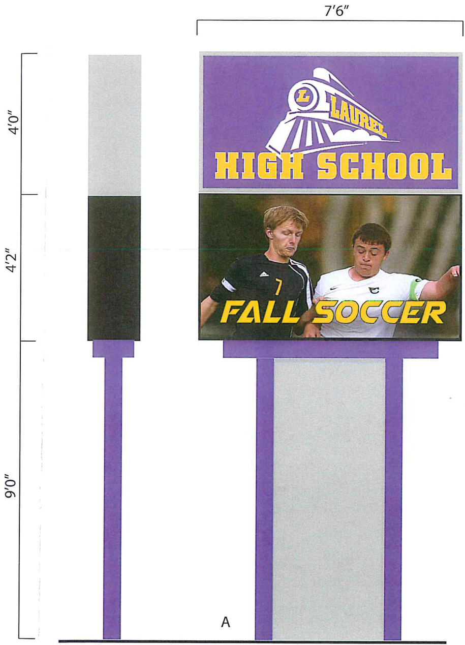
A FABRICATED GALVANEAL GABINET AND RETAINERS, FILMED TUFFAK FACES.ILLUMINATION WHITE LEDS.. NEW GS6 10MM 108X216 RGB MESSAGE CENTER,PAINTED GALVANEAL END FILLERS.6" PAINTED SQ.TUBE ON EXISTING BOLT BASES.PAINTED PAINTEDALUMINUM FILLER.
