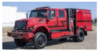
Army 2 ½ ton with a Type 3 or 4 Brush Truck (125-250 gpm pump; 500-750-gallon tank).
