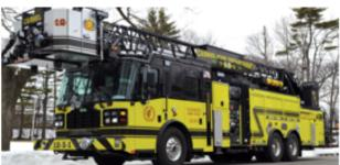
Costs are for the addition of a quint. A quintuple combination pumper, or a quint, is a firefighting apparatus that serves the dual purpose of an engine and a ladder truck. Quintuple refers to the five (5) functions that a quint provides: pump, water tank, firehose, aerial device, and ground ladders. Cost is the estimate for a quint aerial 95' – 103' with a high capacity/1500-2000 GPM
