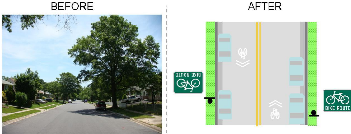
Figure 24: Before and After Signage/Striping Improvements for White Way.
