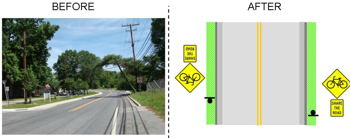
Figure 26: Before and After Signage/Striping Improvements for Bowie Rd.
