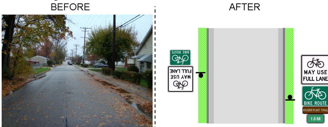
Figure 11: Before and After Signage/Striping Improvements for 9th St.
