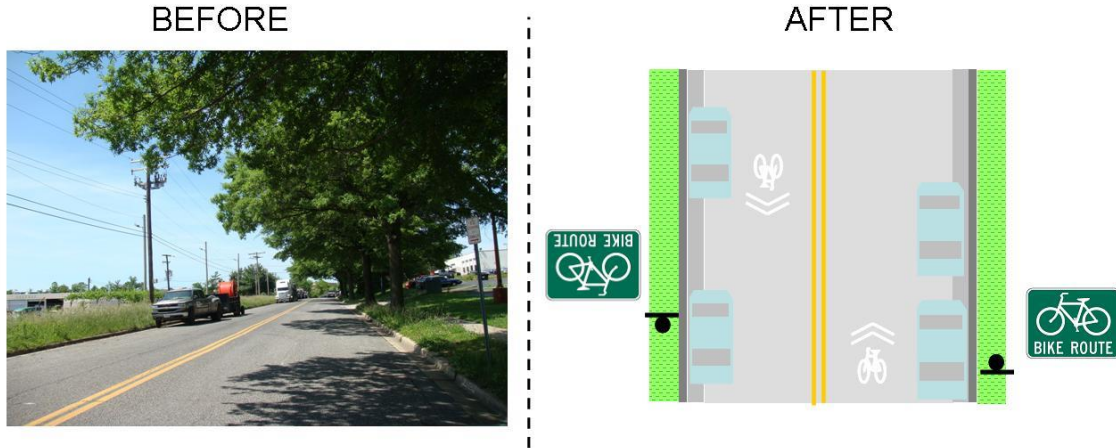
Figure 22: Before and After Signage/Striping Improvements for Staggers Lane
