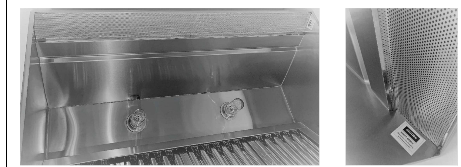
IPS (Internal Perforated Supply) slows air to assist in capture and containment
