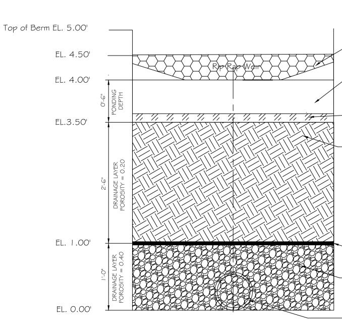
Bioretention Underdrain Layers
