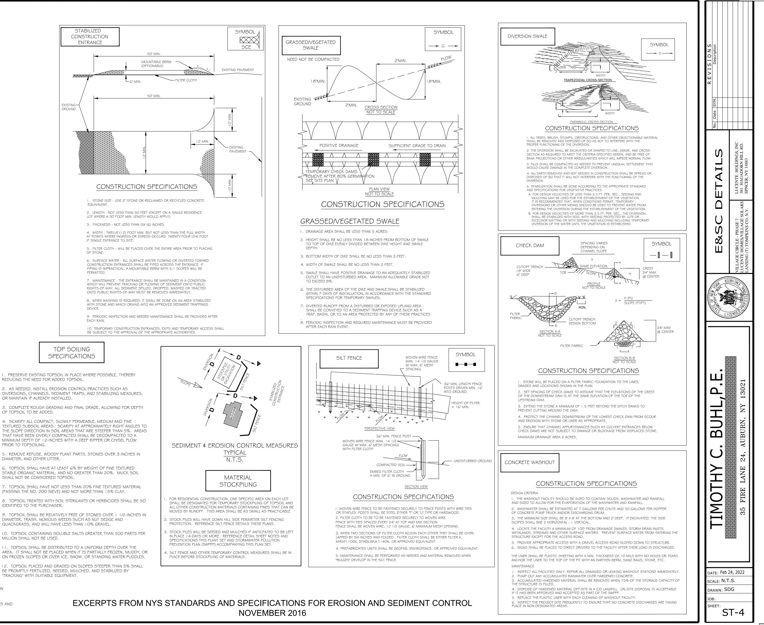
I. PRESERVE EXISTING TOPSOIL IN PLACE WHERE POSSIBLE, THEREBY REDUCING THE NEED FOR ADDED TOPSOIL.
