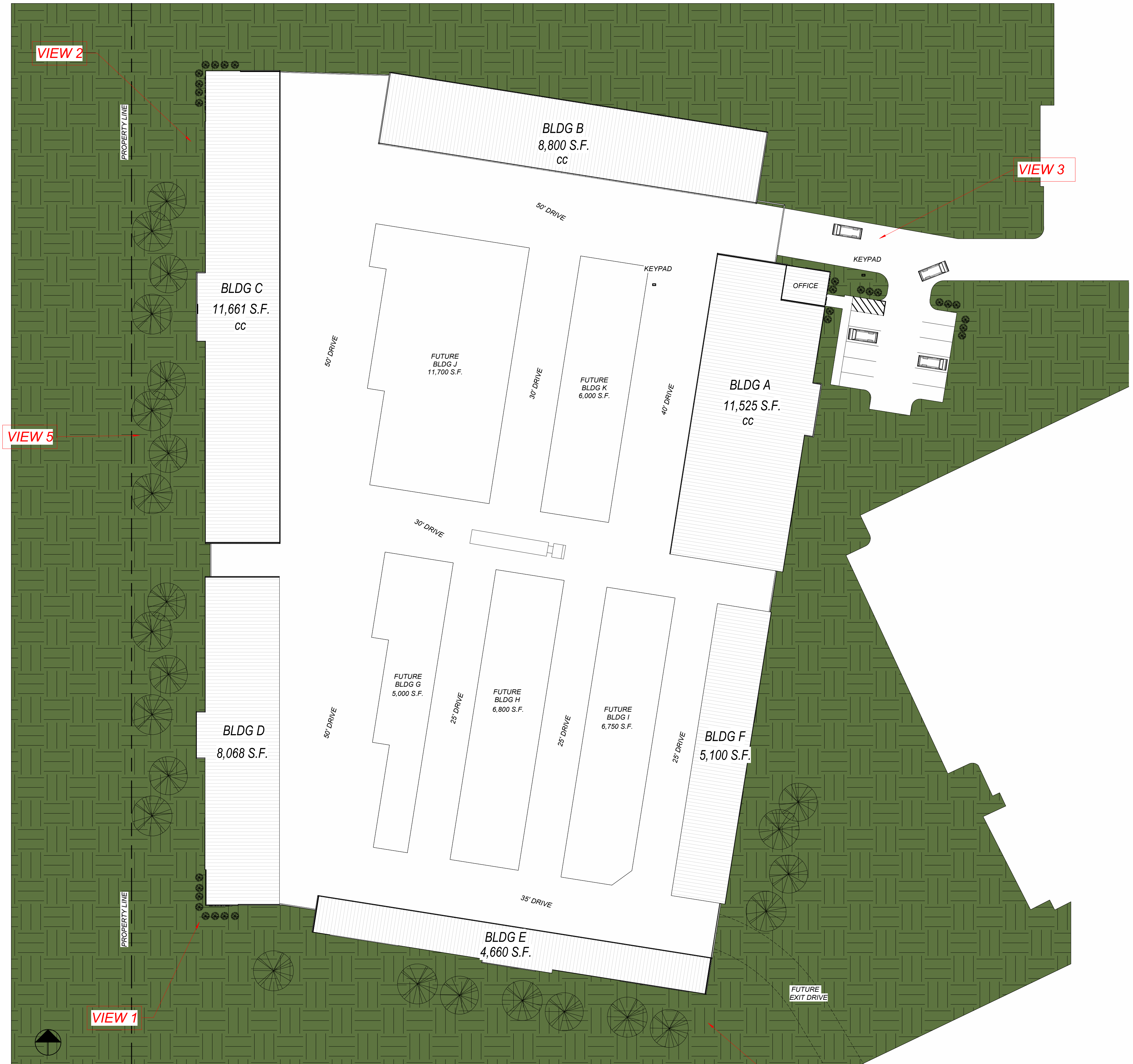
1 ARCHITECTURAL SITE PLAN - 49,814 S.F. PHASE 1 1" = 30'-0"
