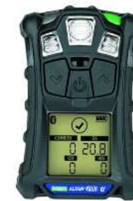
Gas Monitors for All Trucks
