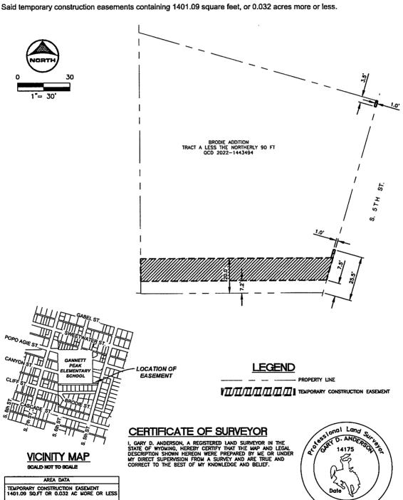
TEMPORARY CONSTRUCTION EASEMENT FREMONT COUNTY, WYOMING
