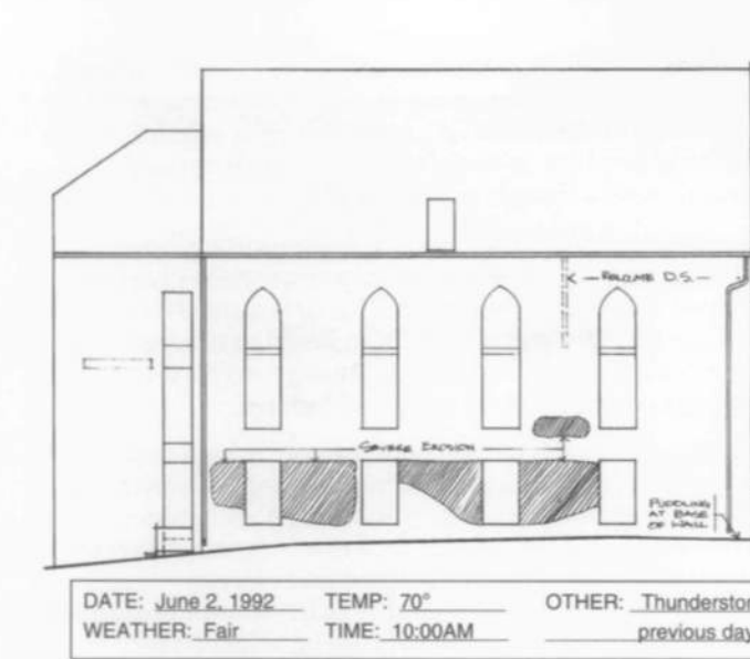
Fig. 13. Using sketch plans and elevation drawings to record the moisture damage along with the date, time, and weather conditions will show how moisture is affecting buildings over time. Drawing: Courtesy, Quinn Evans Architects.
