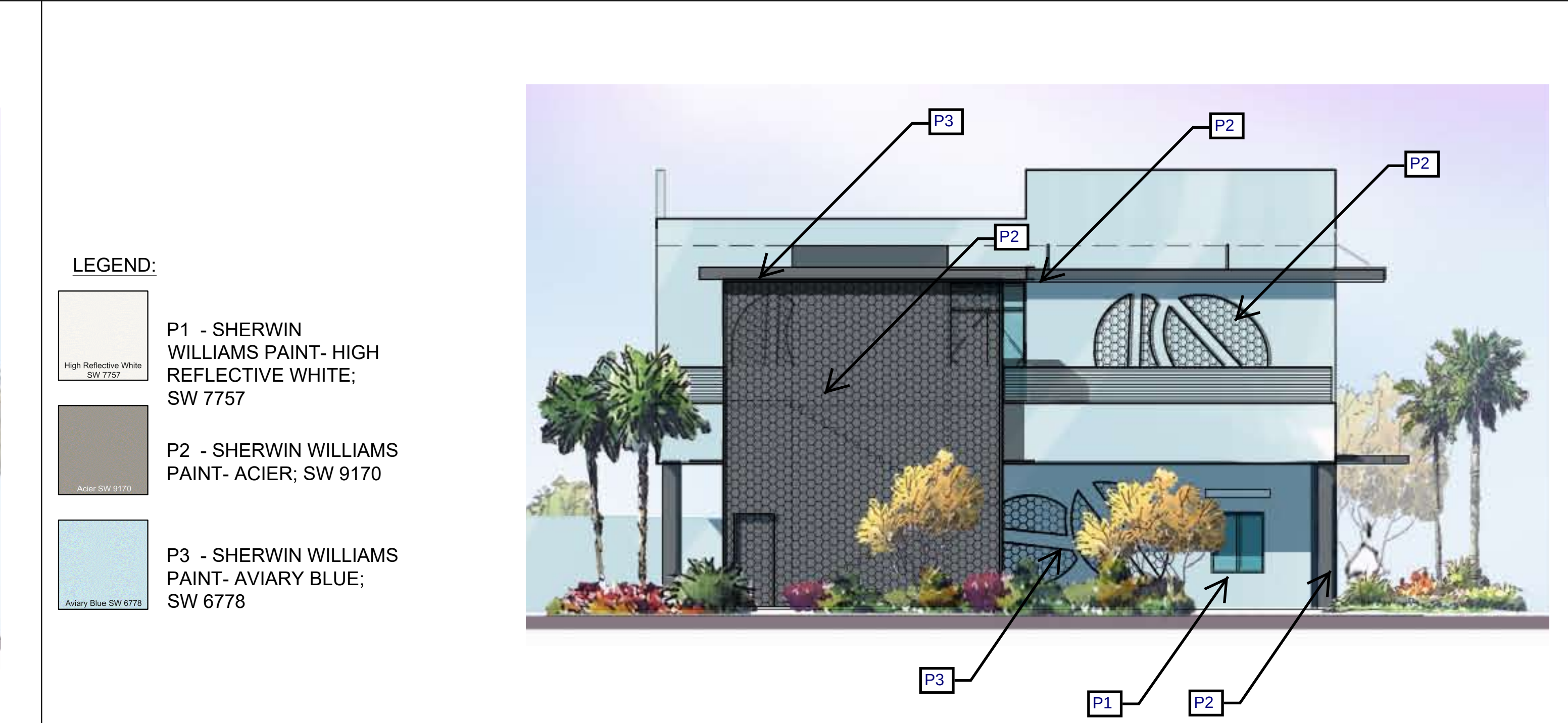
4 NORTH EXTERIOR ELEVATION SCALE: 1/8" = 1'-0"
