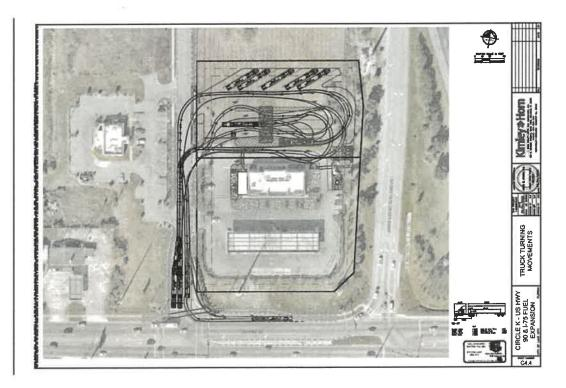
Below is a second drawing of the Truck Turning Movements, which depicts tractor trailer rig access to the high flow diesel pump service bays and alternative egress by exiting through the existing Circle K parking lot and automobile service station area.
