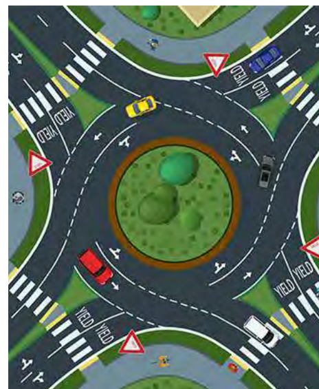
Illustration of a multilane roundabout. Source: FHWA
