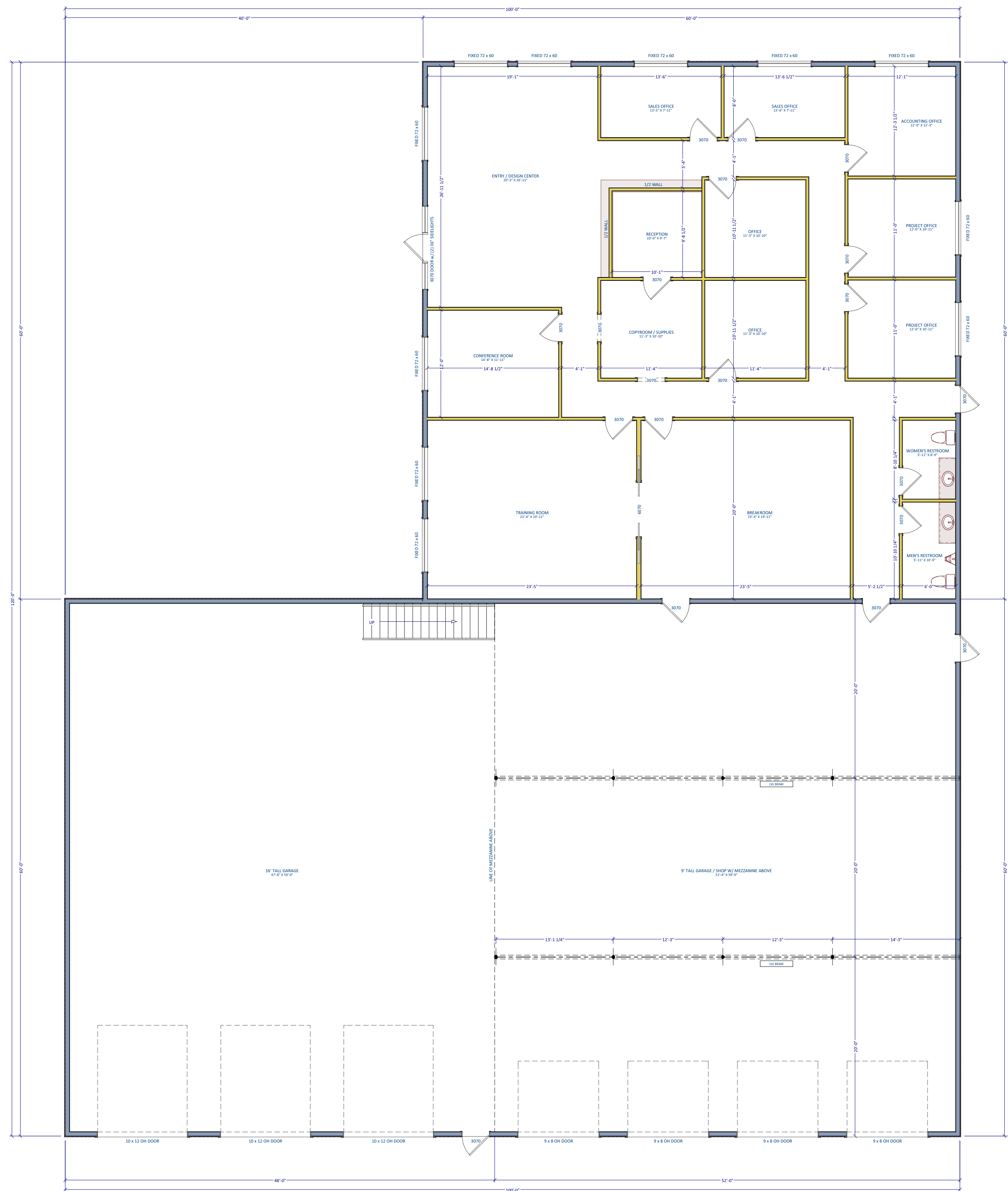
1ST FLOOR PLAN 1/8" = 1'-0" (22x34) Floor Square Footage: --- Garage Square Footage: --- Screen Porch Square Footage: N/A 10'-1 1/8" Wall Heights (u.n.o.) at Offices 10'-0" Wall Heights at Shop 84" Header Height (u.n.o.) Dimensions are Framing to Framing Headers sized by Supplier
