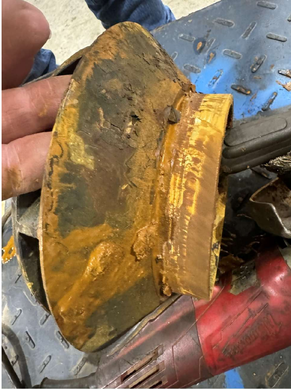
Bottom Side Skirt of the impeller with debris and wear that would not allow for standard removal leading to extra time and measures to salvage and re-use.
