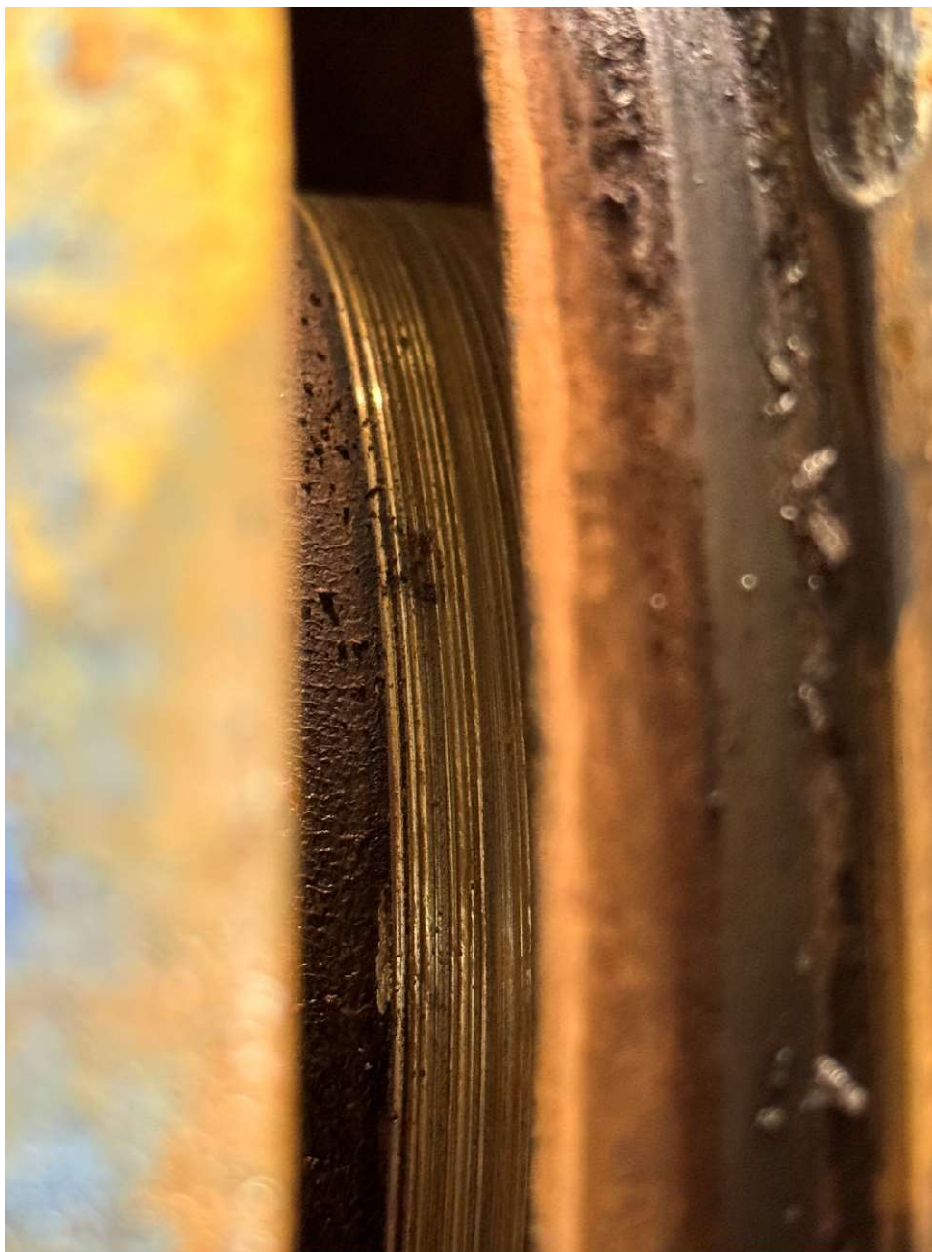
Picture between intermediates showing wear on impeller skirt.
