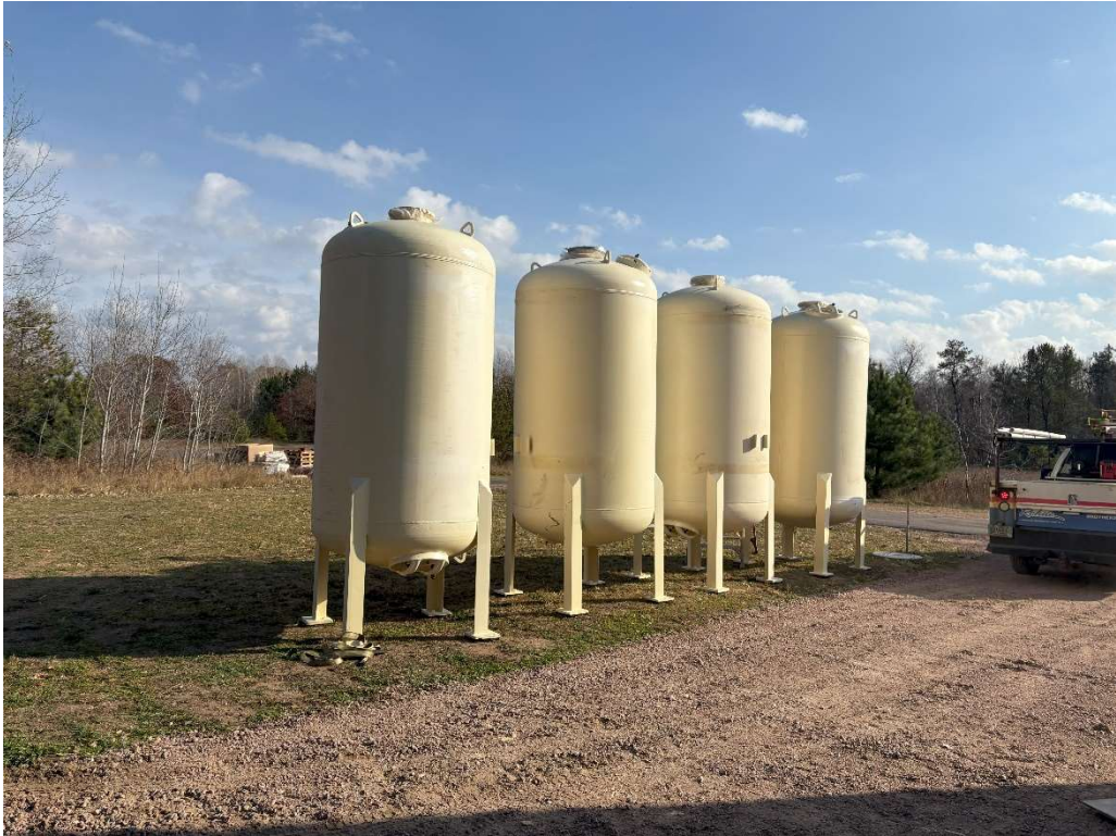
Vertical Pressure Vessels on site.
