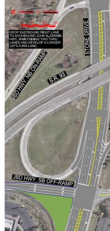
Figure 4. EB Lane Reduction on Stone Drive to allow additional storage at EB Left Turn onto John B Dennis Hwy
