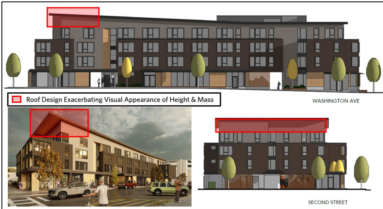
Figure 6: Roof Design Exacerbating Visual Appearance of Height & Mass
