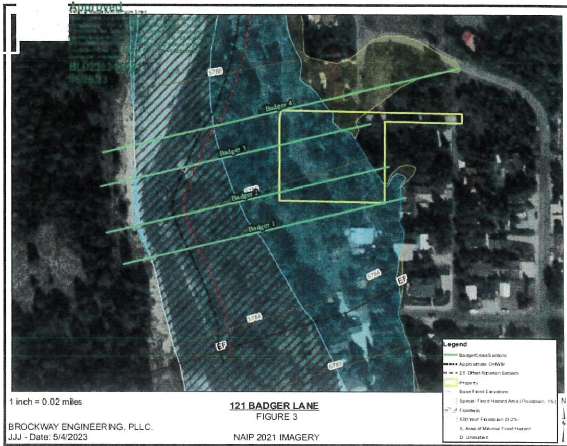
Figure 4. Hydraulic model cross section layout showing model does not capture proposed driveway grading in area of interest. Source: Brockway Engineering, PLLC.
