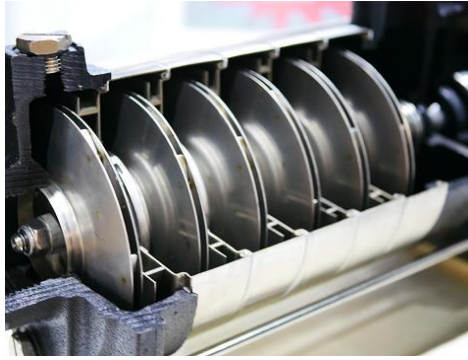
Figure 4. Typical Centrifugal Blower Cross-Section
