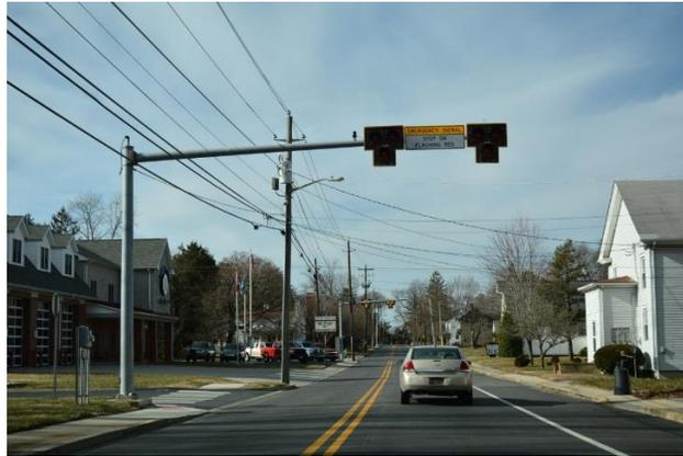
STC optically-activated fire station warning signal
