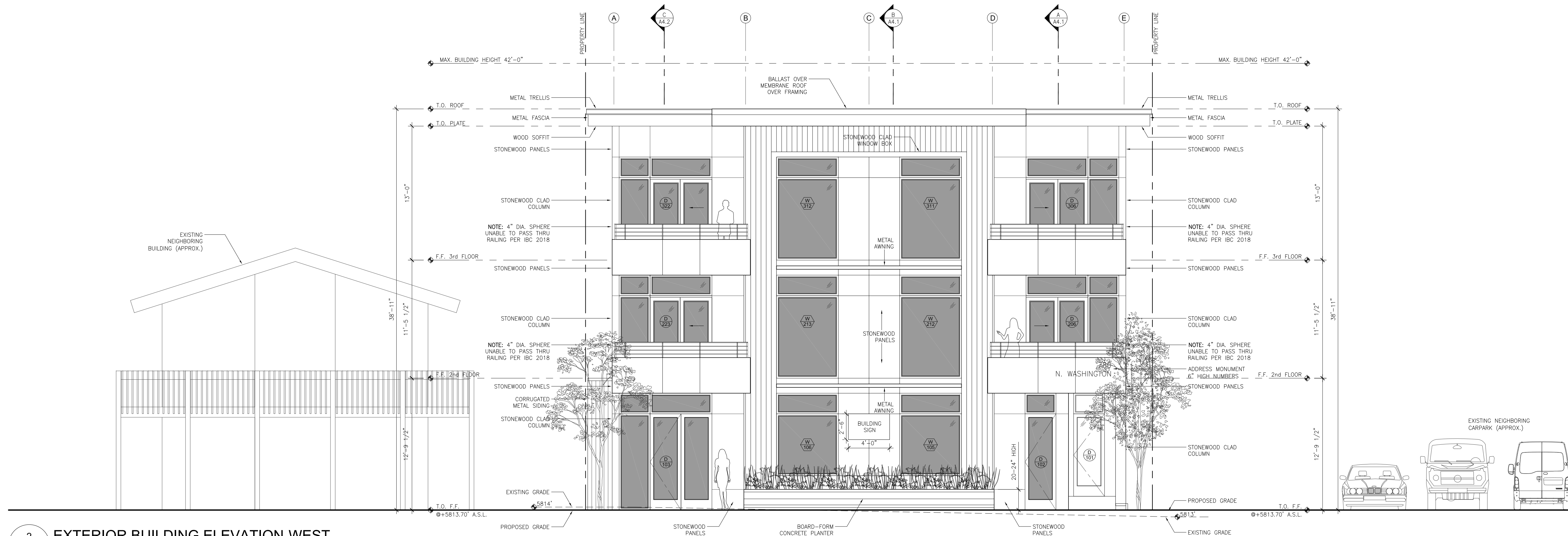
2 EXTERIOR BUILDING ELEVATION-WEST A3.2 SCALE: 3/16" = 1'-0"
