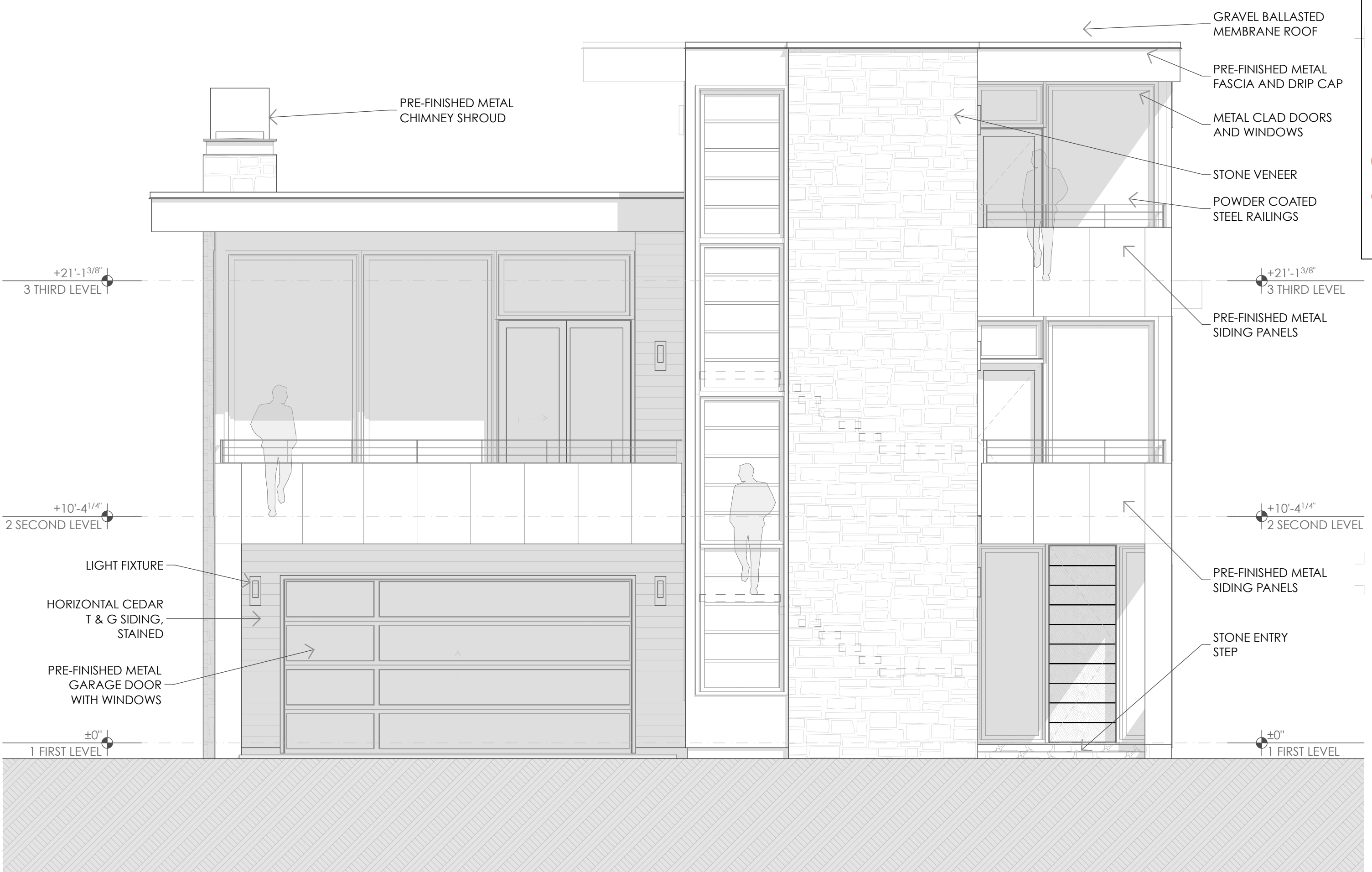
FRONT ELEVATION ③ SCALE: 1/4" = 1'-0"
