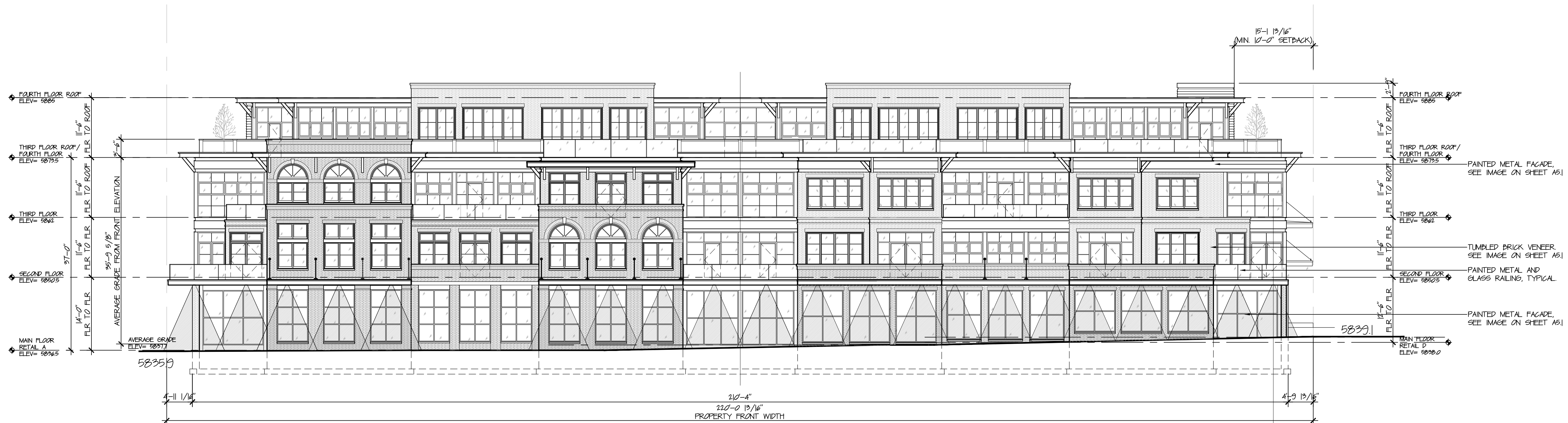
1 FRONT ELEVATION - LIGHTING SCALE: 3/32" = 1'-0"
