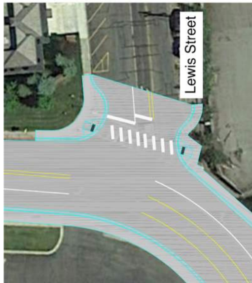
Figure 21. Example Bulb-outs at Lewis Street
