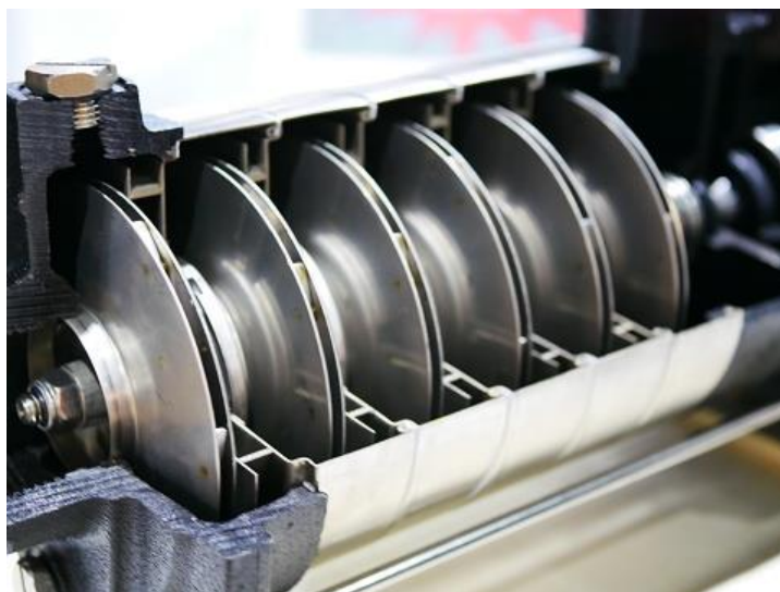
Figure 4-4. Typical centrifugal blower cross-section
