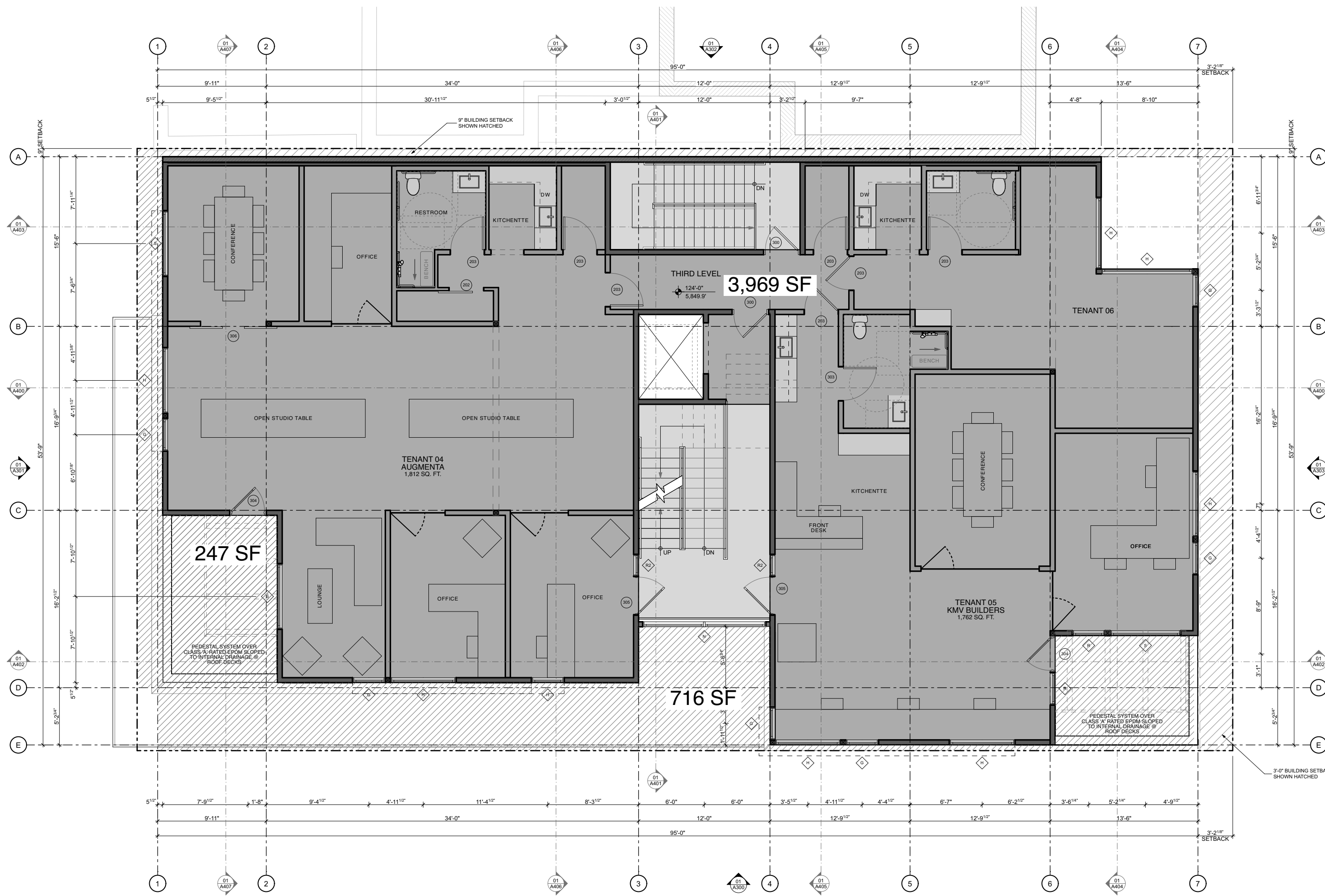
3RD LEVEL PLAN SCALE: 1/8" = 1'-0"
