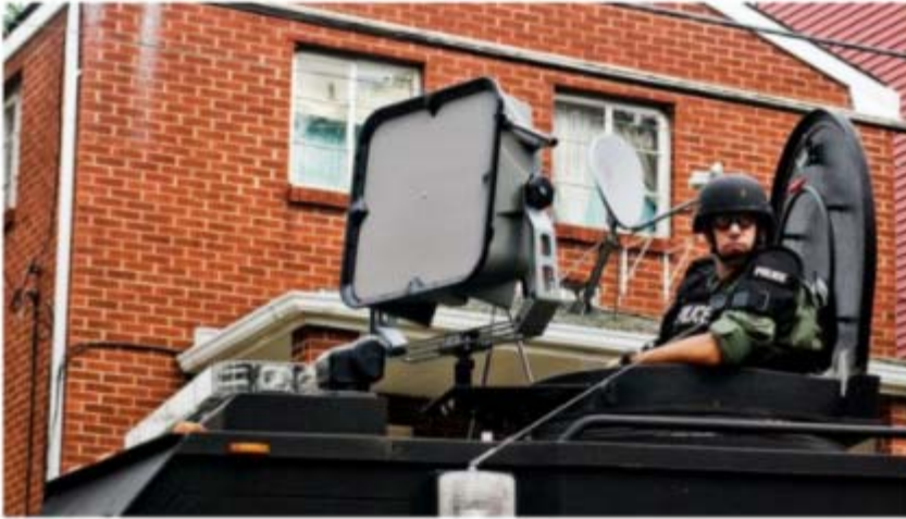
A long range acoustic device in use during the 2009 G20 protests in Pittsburgh, USA. Image: https://www.flickr.com/photos/magnum-photos/10000000000/ (CC BY-NC-SA 2.0)
