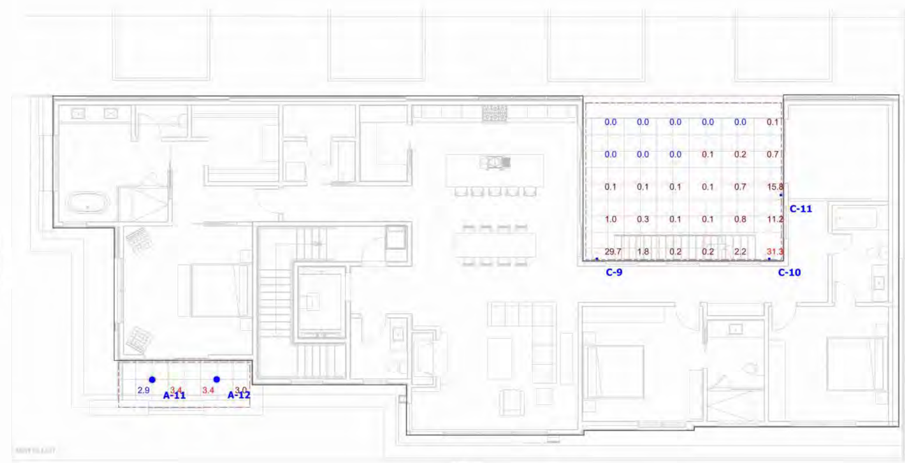
THIRD FLOOR PLAN - EXTERIOR LIGHTING
