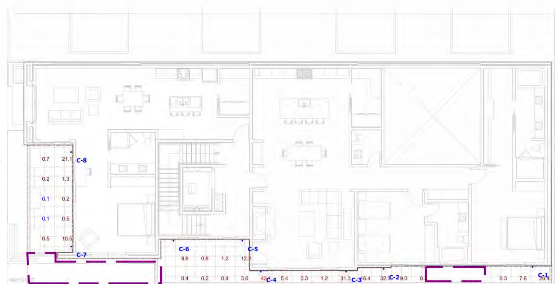
SECOND FLOOR PLAN - EXTERIOR LIGHTING
