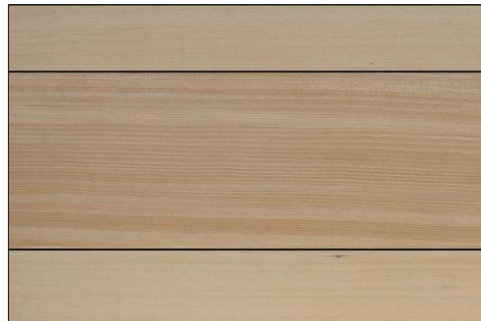
EXTERIOR FINISH 5 (EF-5): EXTERIOR WOOD SOFFIT. RESAWN TIMBER CO. LEWIS WESTERN HEMLOCK
