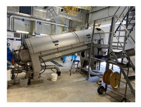
Figure 5-5. Screw press at the City of Hailey's Woodside WRF
