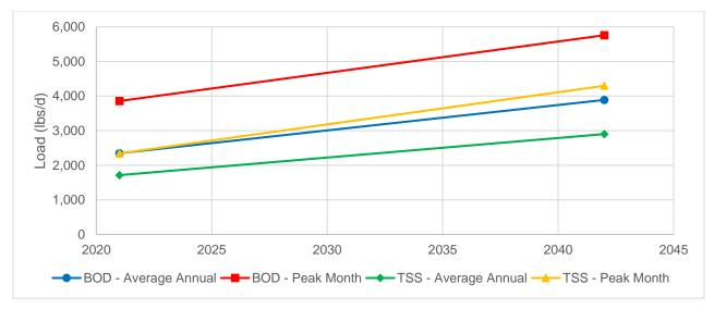
Figure 2-3. Planning period projected wastewater loads
