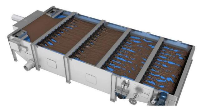
Figure 5-4. Gravity belt thickener
