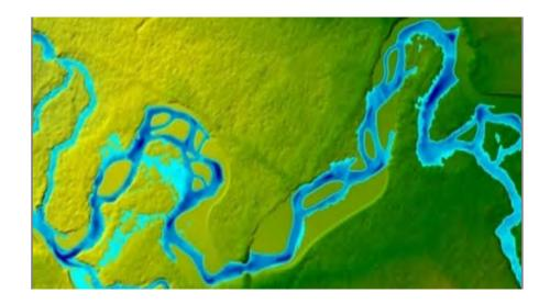
Proposed condition hydraulic depth model illustrating narrower width, many side channels, increased number of pools (dark blue areas) and overall increased depth variability at the 1.25-year flow.
