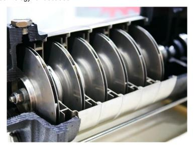
Figure 4-4. Typical centrifugal blower cross-section
