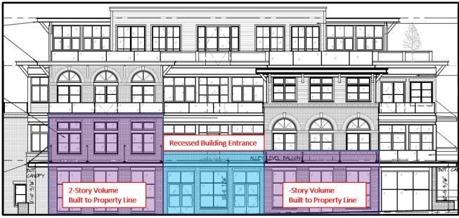
Figure 4: Main Street Building-Mass Modulation
