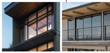
ALUMINUM WINDOWS AND DOORS - powder coated extruded aluminum with Low "E" insulated glass.
