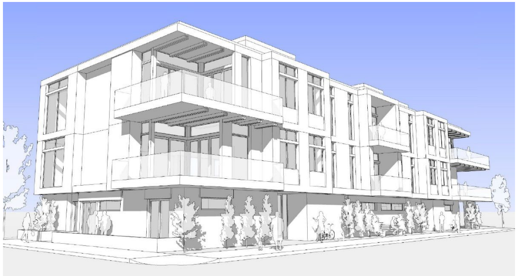
Figure 4. Roof overhangs exacerbating bulk of building
