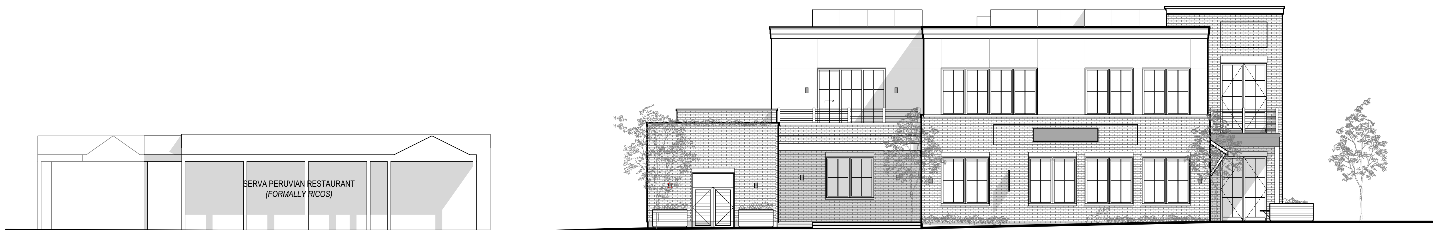
3 ELEVATION: SOUTH (WITH NEIGHBORING BUILDING) SCALE: 1/8" = 1'-0"
