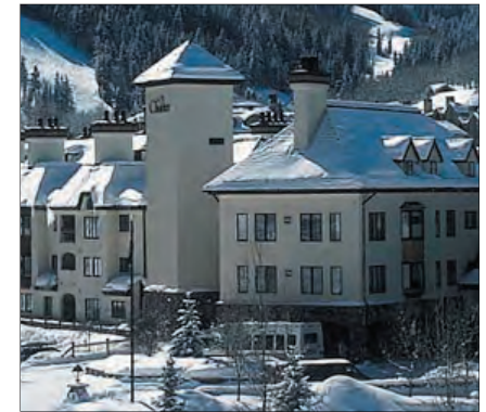
Provide gateway elements, such as towers or other prominent features, at corner locations where appropriate.
