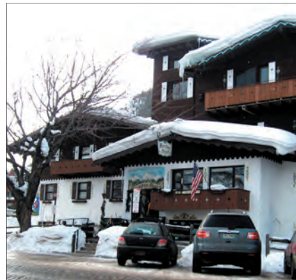
Use varied heights of building masses to reduce the perceived building mass and create visual interest in the building form.
